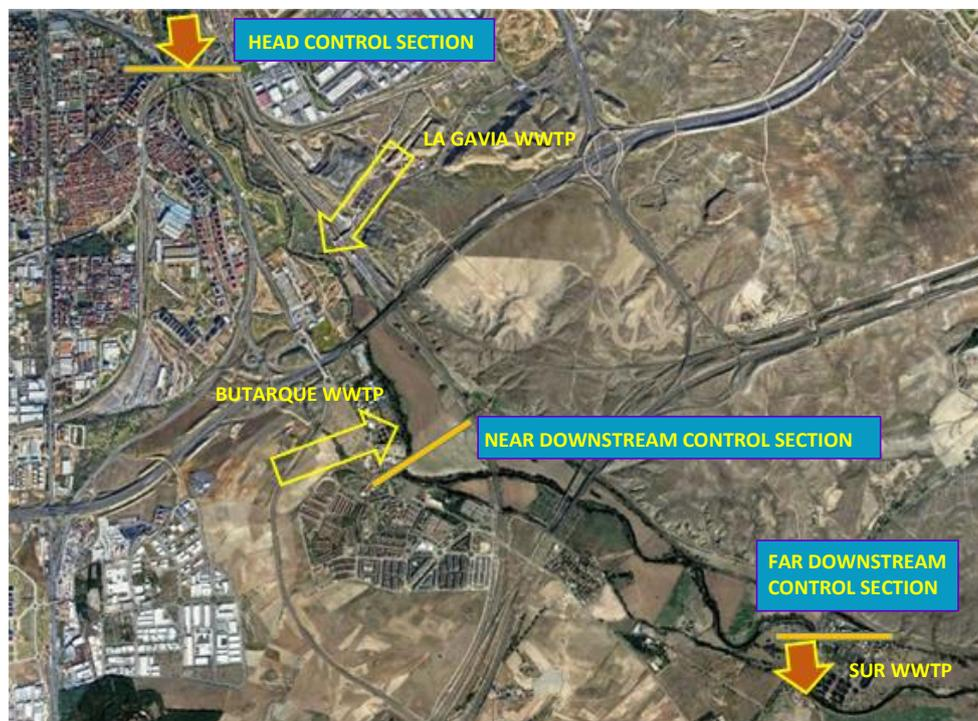
Figure 20 : Planned river quality control sections in Manzanares river
