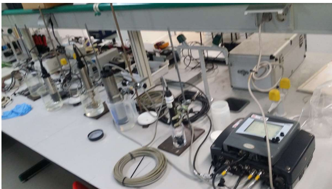
Figure 25. HAC sensors being calibrated in Universidad de la Coruña laboratory
