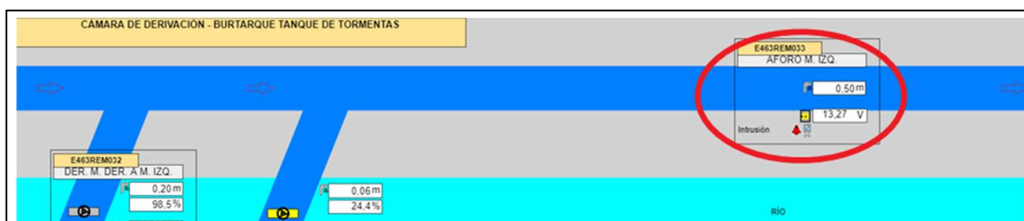
Figure 10. CYII SCADA's view of the existing sensor E463PNC064_NCA located in MI interceptor downstream the pilot area.
