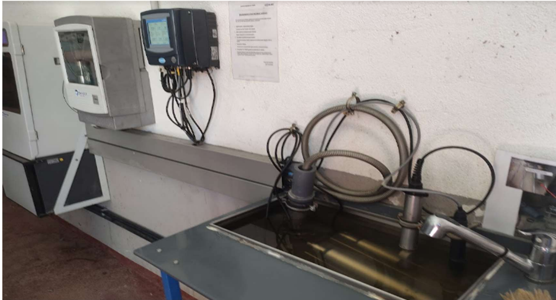
Figure 23. Example of the configuration planned where river water is pumped to a bucket where the sensors are located.
