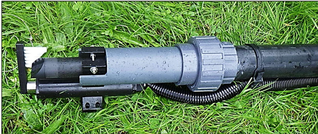
Turbidity sensor and self-cleaning system fixed on the PVC protective pipe
