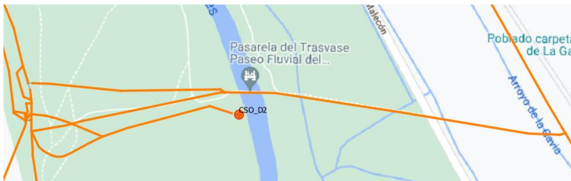
Figure 6.- By pass sewer driving waters from the right margin interceptor to the left one.
