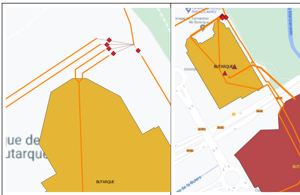
Figure 42.- Actuators controlled in Butarque tank (left zoom to the entrance and by pass gates from the right margin interceptor)
