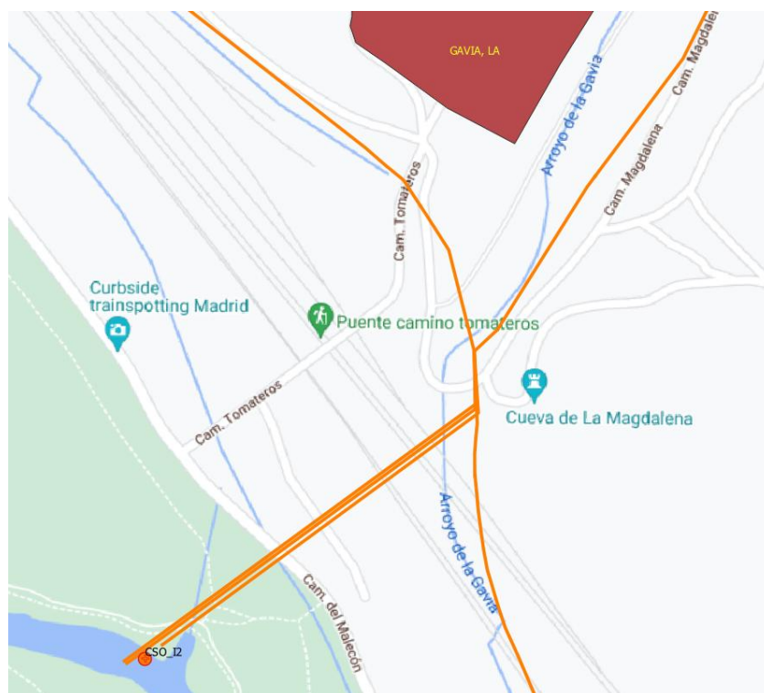
Figure 21.- Aliviadero Sur discharging point to the river and the location of the weir chamber between
