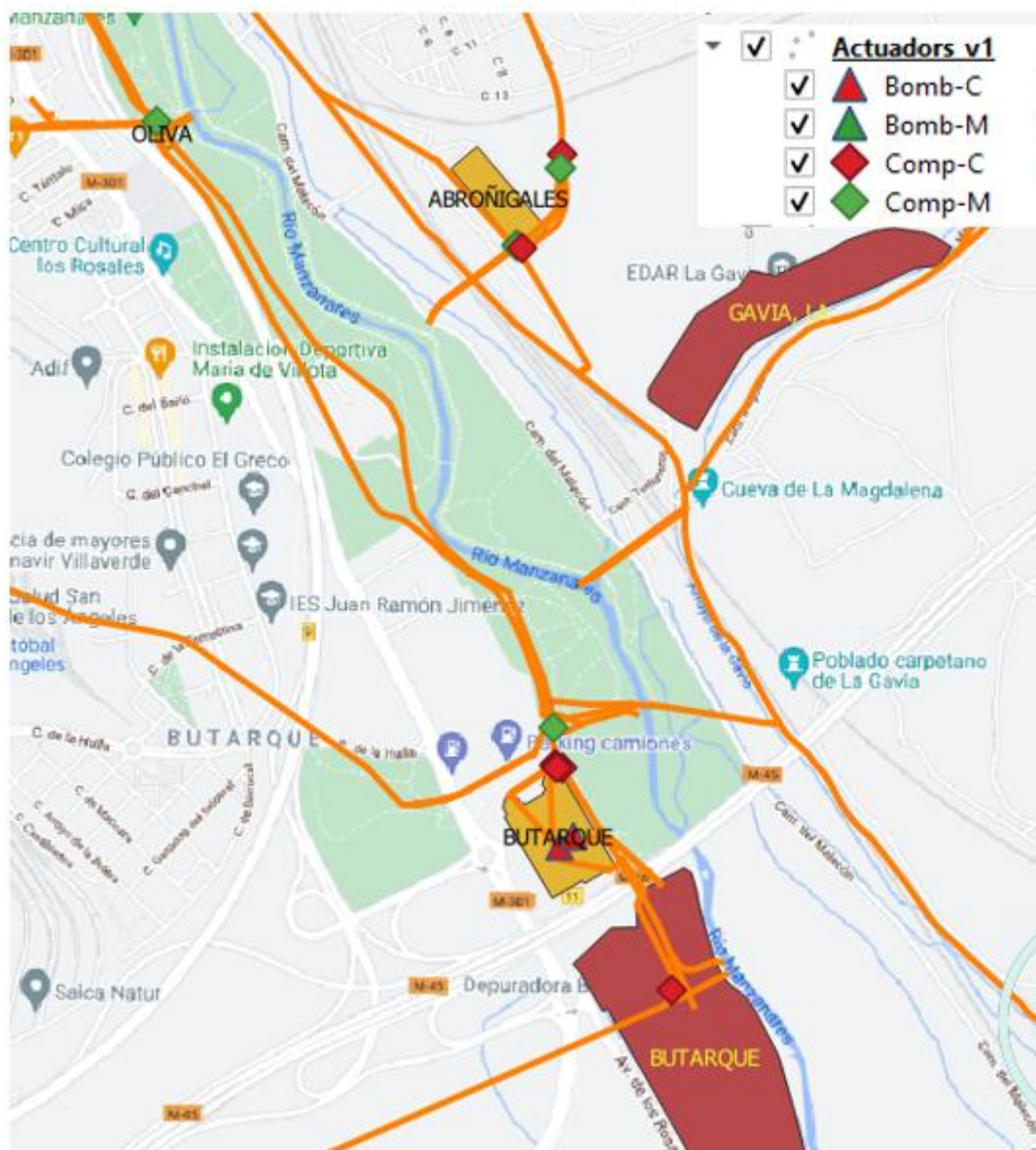
Figure 41.- General view of the actuators in the pilot site. Triangles are the pumps while diamonds are the gates. Also green ones are the ones that will be monitored in the project, while the red ones are the ones that will be fully controlled by Rubies algorithms
