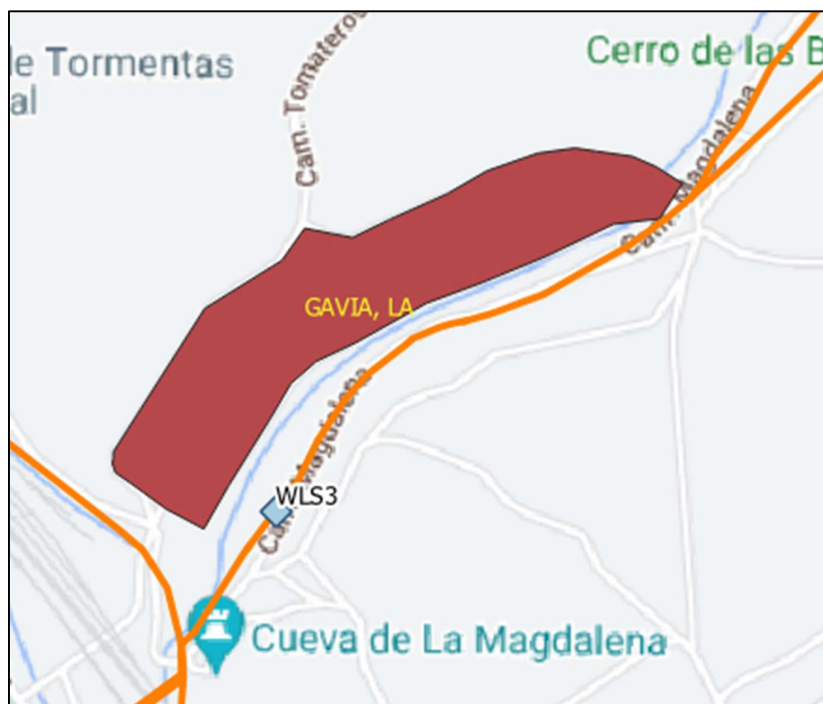
Figure 7. Optional future location of the water level sensor in La Gavia collector
