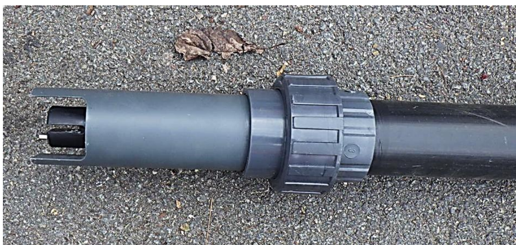
Figure 9 Conductivity sensor fixed on the PVC protective pipe
