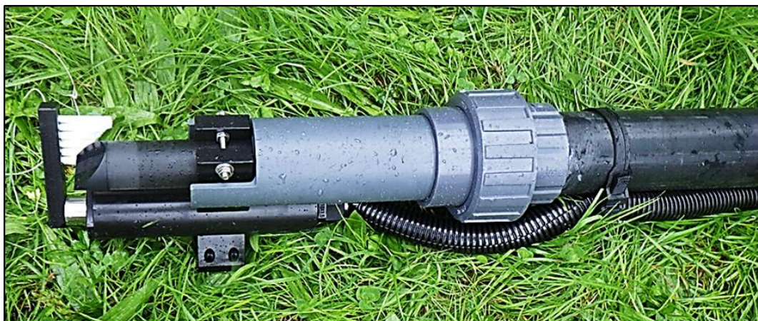
Figure 8 Turbidity sensor and self-cleaning system fixed on the PVC protective pipe
