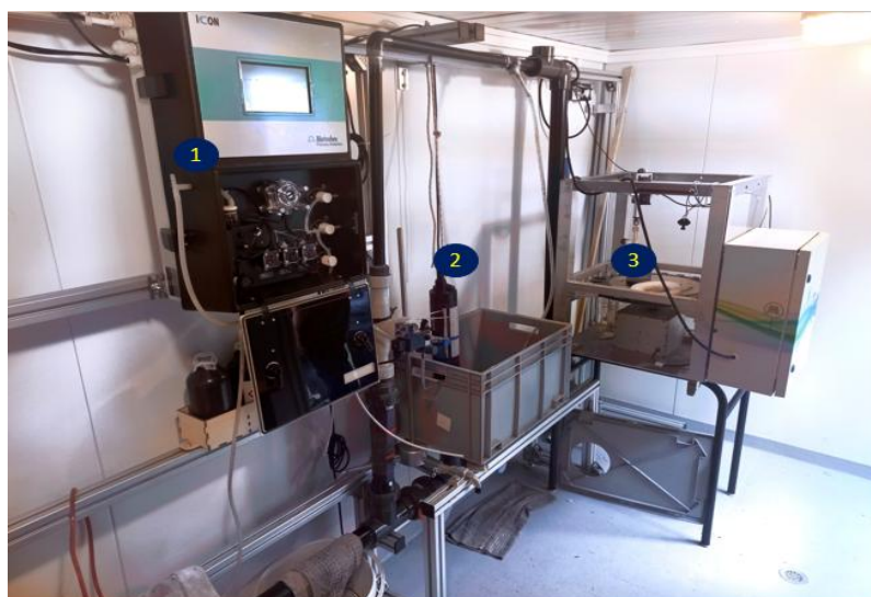
Figure 4 : Apparatus deployed in the mobile laboratory for high frequency measurements: 1) an ammonium analyser; 2) a multi-parameter probe; and 3) the filtering sampler "FILEAU".
