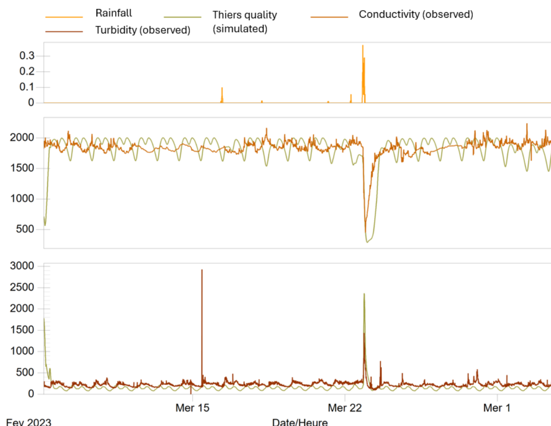
Figure 13: Turbidity and conductivity water quality simulation results at Thiers during dry and wet weather conditions, used to estimate pollutant loads through correlation relationships.
